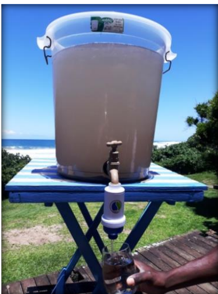
Figure 8: Rural Household Water Treatment System/Hand Washing Station
