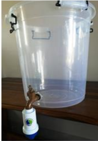
Step 5 - Attach the filter/purifier to the plastic tap
